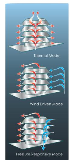
The purpose of venting the roof is to improve the living environment in the rooms below.
