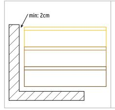
• The finishing structures of the wood cladding profiles should be worked out so as to leave working spaces. All endpoints of the cladding profiles (wall, ground etc.) should have at least 2 cm space.
