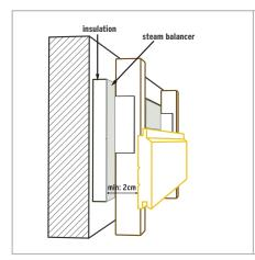
• The material used as steam balancer should completely cover the rockwool and without any space between the material and the rockwool. But a minimum distance of 2 cm between the steam balancer and wood should be left.
