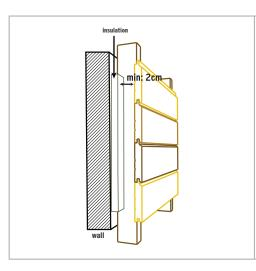
• Underconstruction dimensions should be determined so as to leave 2cm air pocket between the cladding profiles and the supporting surface.
