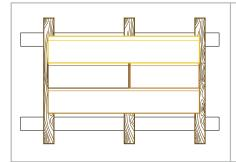
• The head parts of cladding profiles should definitely be aligned with underconstructions.
