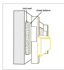
• In case the material used for heat and/or sound insulation is rockwool, steam balancer (tyvek or equivalent) should be applied on rockwool in order to prevent the transpiration caused by the condensation resulted from the indoor and outdoor temperatures .
