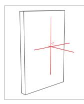
• The surface to be cladded should be gauged and plumbed.
