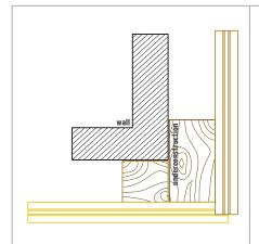
• Merging points on the corners should definitely be supported with underconstructions on the back. Working spaces should be formed at the front and rear of the corners.
