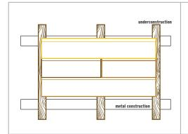
• In case a construction material (aluminum, steel, galvanized iron etc.) other than wood is used, it is recommended to use a wood carcassing on top of this construction material to avoid different working principles.
