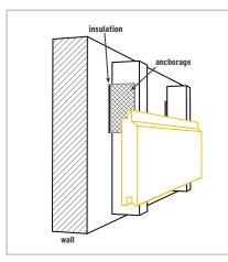
• Use of insulated anchorage material is suggested in order to prevent heat bridge.
