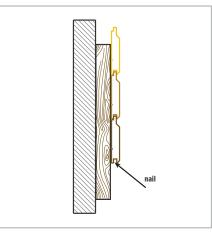
• Stainless nails shot with air gun can be used during the installation of cladding profiles. The nails should be driven invisibly through the grooves of wood.
