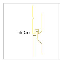
• There should be at least 2 mm working space at the T&G and back merging points of cladding profiles. To do that, spaces can be formed on the front merging points of cladding profiles using a pre measured lath.
