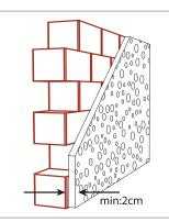
• Minimum 2cm thick rough plaster should have been applied on the brick wall.
